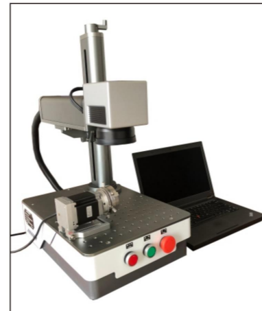
Jewelry small marking machine with electric rotating shaft.
