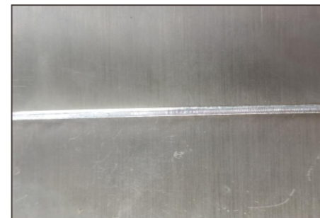
Stainless steel plate splicing
